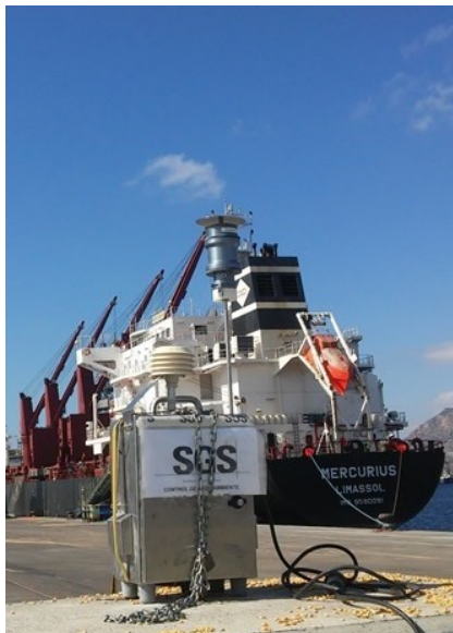
Study on the sulphur particles present in the dust of the bulk terminal of Escombreras expansion, installation of collectors October 2017
