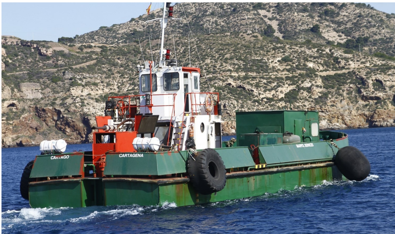
Gabarra Cartago for MARPOL service has a hydrocarbon water treatment plant.
